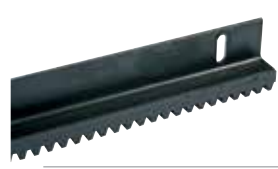
ACS9040 Module 4 STEEL RACK (sect. 22 x 22 mm) with right-angle member (up to 2200 kg) recommended for K500 FAST in 2 m bars per m
