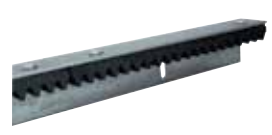
ACS9006 Module 4 RACK (sect. 25 x 22 mm) in Nylon with right-angle (up to 1000 kg) in 1 m bars per m
