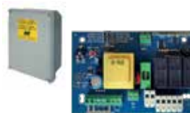
ABJ8042 R-CRX 2.0 control board for 1 BOY with radio receiver 433 MHz. With box IP55. See page 141 and 147
